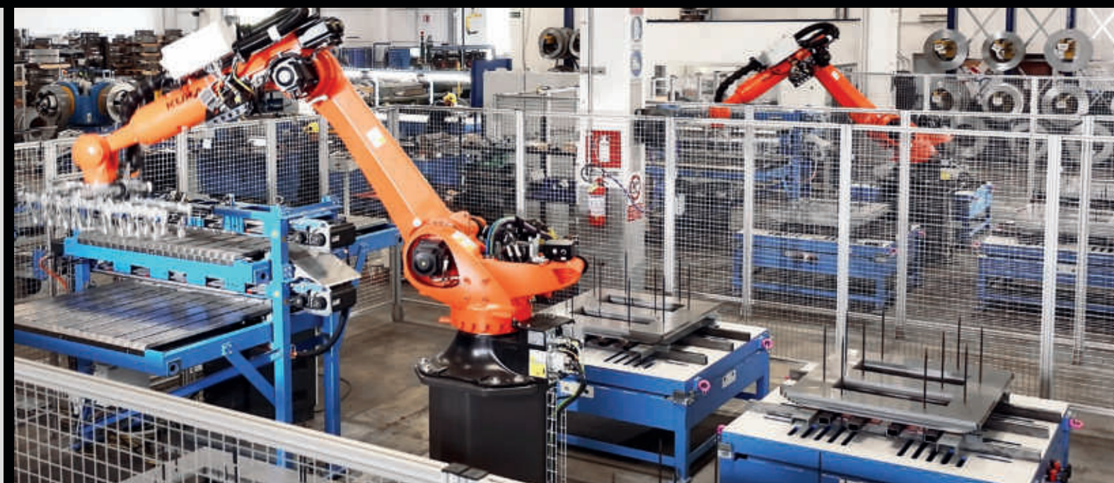
Automatic Cutting and Assembling lines for distribution cores
